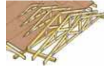
Valley sets as over-framing
